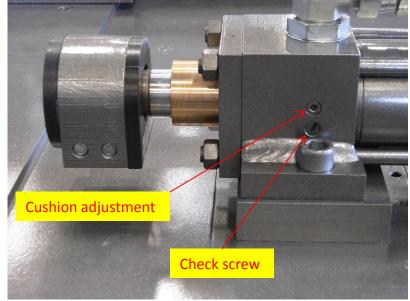
The bottom screw is another internal check, NO adjustment. The Allen style is used to adjust the cushion. With the feed drawer installed adjust so the cylinder is NOT banging at end of stroke. This should be check every six months for correct operation. Failure to do this will resolute in premature cylinder failure. Every cylinder new or rebuilt need this adjust performed.
